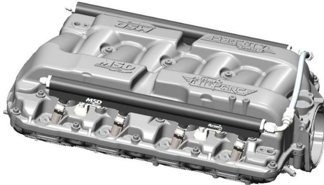
Atomic® billet fuel rails work with the application's OEM injectors and tall EV1/Bosch style injectors (see chart Page 3). **NOTE:** If using tall EV1/Bosch style injectors on LS7 or LT applications, there may be interference on low hoods on Corvettes and similar.
