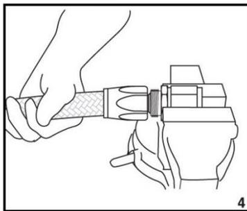
4. Holding the hose and not the socket, push the hose and the socket onto the nipple until the socket threads can be started on the nipple. Holding the hose and not the socket, start the threads and go as far as you can by hand. Depending on the size of the hose, some force may be necessary in this part of the operation.
