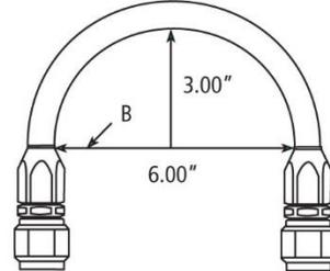
Minimum bend radius is measured on the inside bend of the hose. To determine minimum bend, divide the total distance between ends (B length) by 2. For example, B=6, minimum bend radius=3.
