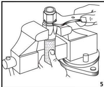
5. To complete the assembly it doesn't matter whether the nipple or the socket is held in the vise. Holding one or the other in the vise and using a suitable wrench on the other, tighten the socket onto the cutter threads until the socket is within .060" of bottoming on the nipple. Do not use an adjustable or over-size wrench or you will damage either the nipple or the socket.
