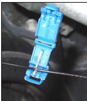
Figure 9 (T-Tap connector installation)
