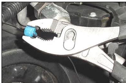
Figure 10 (Close T-Tap connector)
