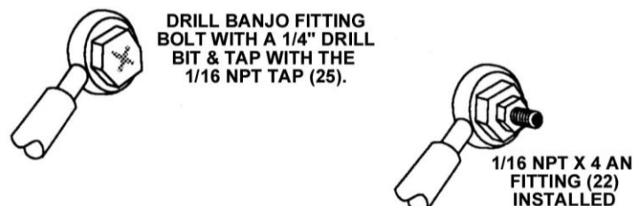
Figure 8 Schematic of "Drilled Out" Banjo Fitting
