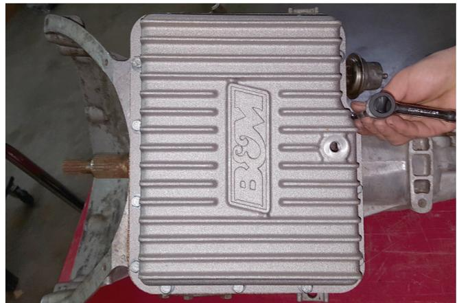
11. Install **drain plug gasket (11)** and **drain plug bolt (10)** into deep pan, tightened to 20-25 ft-lbs.
