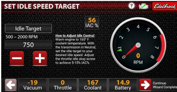
17. The Setup Wizard is now complete and engine tuning can commence. Refer to the Forced Induction tuning guide on Page 31.
