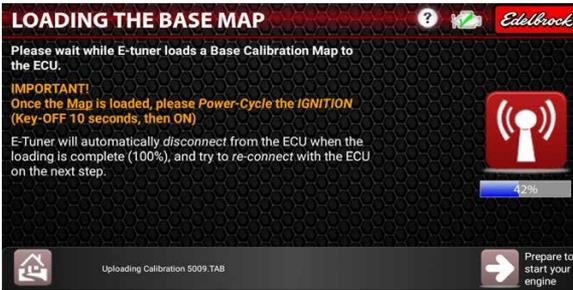
14. Read the important warning then tap the check mark to continue. **Do NOT start the engine or drive the vehicle until prompted to do so.**
