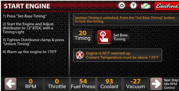
b. Start the engine and adjust the throttle body screw, as needed, to maintain idle. **Do NOT drive the vehicle yet.**
