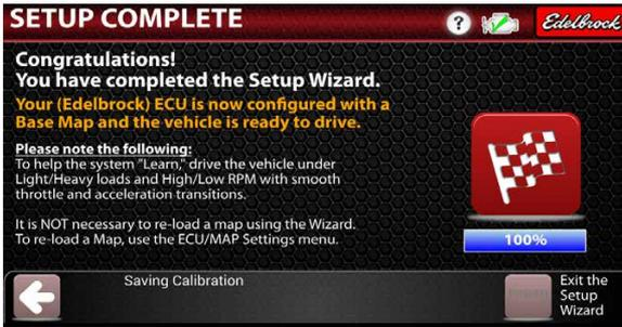
**TIP:** The key to driving your vehicle initially with the Pro-Flo 4 EFI System is to employ smooth slow throttle transitions and accelerations. Try to drive the vehicle in a manner that covers all conditions, such as: light load, heavy load, high RPM and low RPM. See page 30 for additional tuning recommendations.
