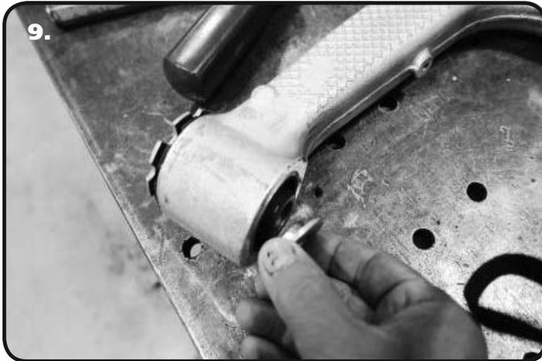
9. Remove the small T-bushing from the inner side of the OEM bushing. This can be done by simply prying them out with a small pry bar.
