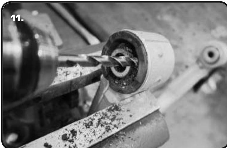
11. Using a drill and 5/16" drill bit, drill the rubber out of the bushing. You can start by plunging several holes around the bushings. Drill as many holes as you can leaving very little rubber. The remaining rubber can be cut out with the drill bit by going in a circular motion around the inner sleeve. Let the drill do the work for you. Remove the inner sleeve when it comes loose.
