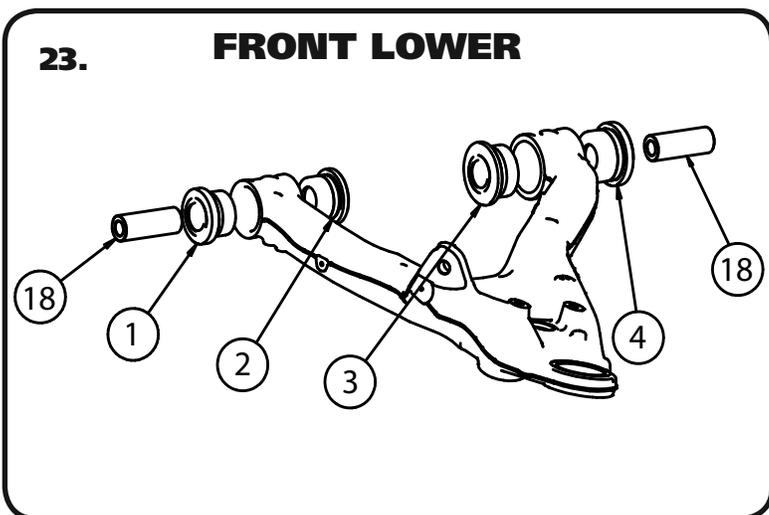
**23. Front Lower** - Using the Diagrams on Page 2 & 3, Insert the correct Bushings in the correct locations using a Bench Vise to push them in. Push the Bushings in followed by the correct Inner Sleeve. The Front Lower uses Bushing[1, 2, 3, 4], and Inner Sleeve[18].
