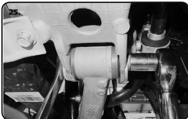
**25.** Tighten each Cam Nut, but first align the mark made on the Cam. Hold the Adjusting Cam Bolt Head in place with a wrench while torquing the Cam nut. Torque the Cam Nut to 125 ftlbs.
