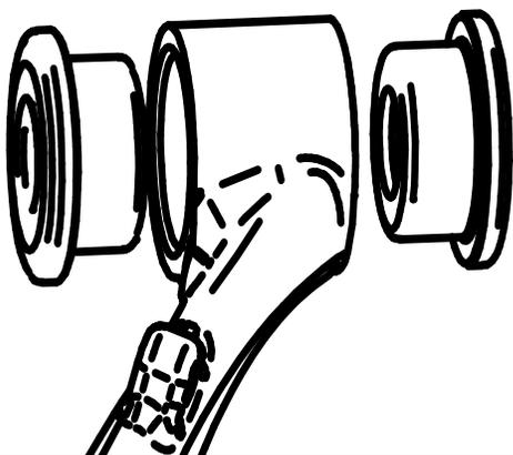
18. Press a set of bushings into each opening of the upper control arm. A bench vise can be used to do this.
