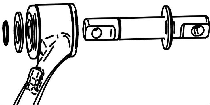
19. Install a Trunnion into each set of Bushings installed in the Control Arm. The Trunnions are inserted with the Shoulder to the outside of the Control Arm. Install a 3/4" Washer followed by a Snap Ring on each Trunnion.
