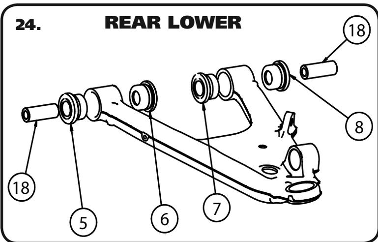
**24. Rear Lower** - Using the Diagrams on Page 2 & 3, Insert the correct Bushings in the correct locations using a Bench Vise to push them in. Push the Bushings in followed by the correct Inner Sleeve. The Front Lower uses Bushing[5,6,7,8], and Inner Sleeve[18].
