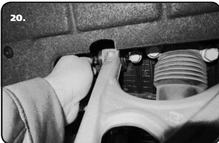
20. Reinstall the Control Arm on the car with any shims back into their previous location. Tighten all Fasteners.
