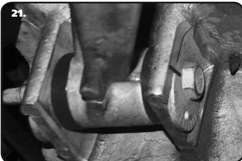
**21.** Before removing the Lower Control Arms, use a **Marker or something similar to mark the Lower Control Arm Adjusting Cams position.** The marks will get the Alignment close, but Ridetech recommends getting the alignment checked after the install is completed.
