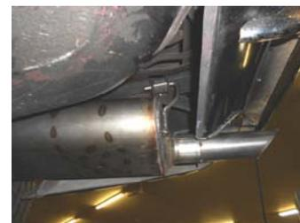
4) Place one of the supplied **HA602** rubber mounts onto the wire hanger of left muffler assembly **842557-356**. Place a provided clamp onto the muffler inlet, then place the assembly onto the back of the mid pipe and slide the two fully together. Support the muffler with a stand. Using a supplied 3/8" bolt, nut, washer and lock washer, bolt the **HA602** hanger to the hole in the frame above the muffler outlet.
