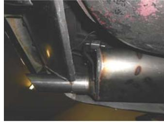
5) Adjust the position of the pipes and mufflers to provide a satisfactory fit. A minimum of 3/4" clearance around all parts of the system must be maintained; while also keeping suspension travel and vibration in mind. Tighten all clamped connections down securely.
