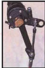
7. Reinstall the shift lever as close to the swivel as possible. Now you could turn the bracket or loosen the large nut and adjust so that the swivel goes into the 5/16" hole that you drilled in the shift arm. Insert the cotter pin in the swivel, tighten the large nut and bolt on the bracket. Do not tighten so much that it squeezes the delrin bushing in the bottom of the column. This could make it hard to shift. Remember, the cable has to be pushed down completely.
