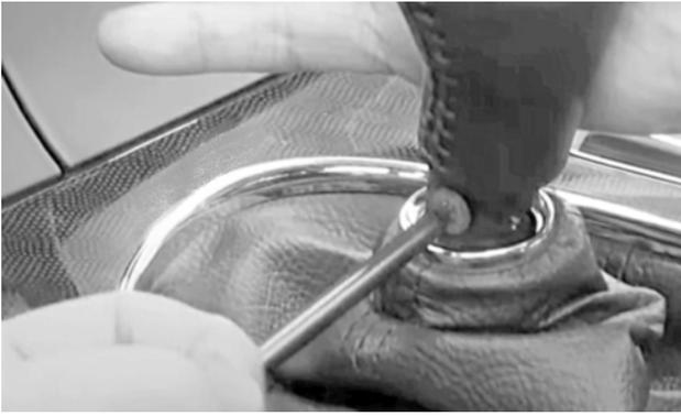
2. Remove the shift knob screw, then lift the knob off of the shift lever.
