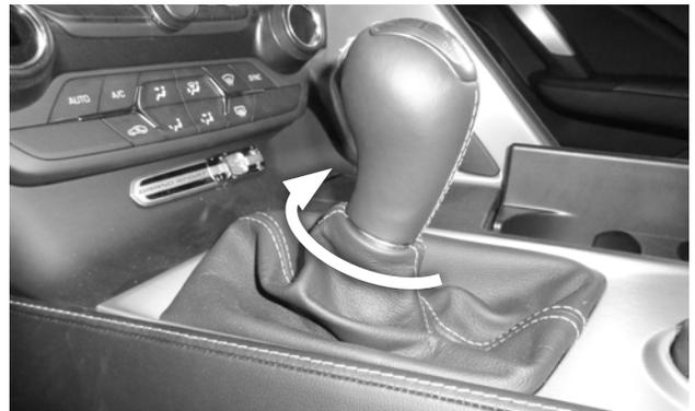
**75. Firmly grasp the chrome ring and turn it 1/4-turn clockwise** to lock it into place on the knob.
