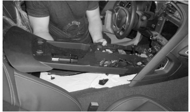
62. Carefully return the console base to the vehicle.
