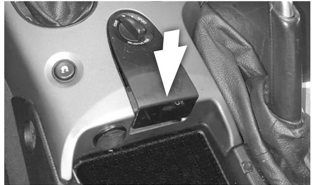
31. EARLY C6 (2005-2007) ONLY: Reconnect any electrical plugs to the half-round panel, then reattach the panel to the front console.
