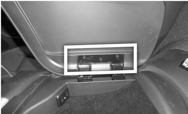
35. **Open the center console lid**, remove the 3 hinge screws, remove the lid, and close the hinge.
