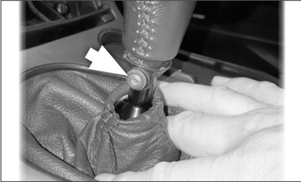
**Place the knob on the shift lever.** Apply medium-strength thread locker to the **6mm screw**, and secure the knob to the lever at the larger (bottom) screw hole.
