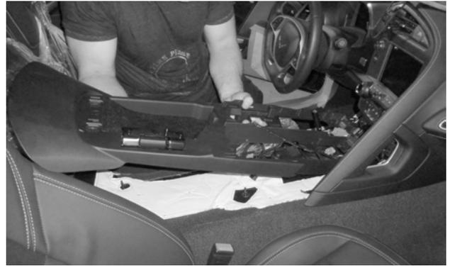
49. Carefully remove the console base and set it aside.
