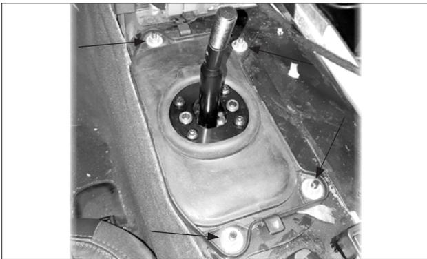
60. Reinstall the rubber dust boot using the 4 stock nuts.
