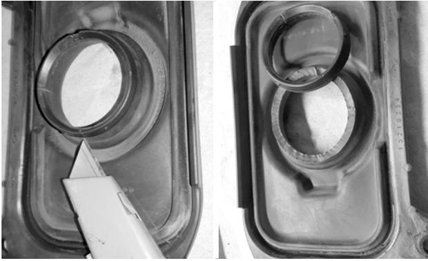
59. Use a sharp, new blade to cut the hard plastic edge off the bottom of the rubber dust boot, to allow the boot to fit around the shifter base.
