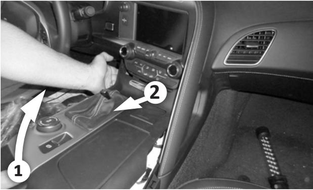
41. Lift up on the back and sides of the console panel, then gently pull rearward to free its front end from the console base.
