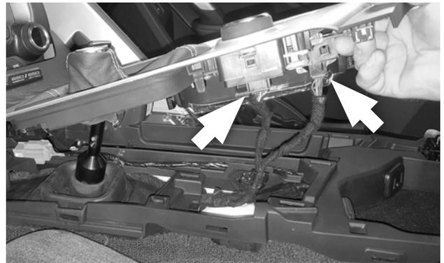
70. Reconnect the parking brake and Mode Select plugs, and check the security of the connections.
