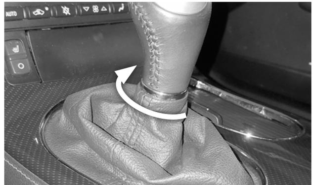
**Then firmly grasp the chrome ring and turn it 1/4-turn clockwise** to lock it into place on the knob.
