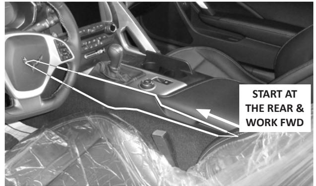
37. **Starting at the rear of the left side trim panel and moving forward**, detach 5 friction clips to remove the panel from the console.
