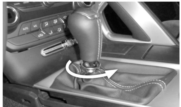
38. **Separate the leather boot from the shift knob** by firmly grasping the chrome collar, turning it 1/4 turn counter-clockwise, and pushing it down to expose the screw.
