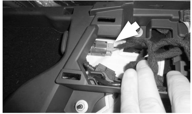
68. Reconnect the 12v power plug, and check the security of the connection.
