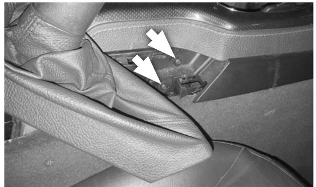
6. On the left side of the parking brake, feel down through the boot, and separate the 2 friction clips from the console base. Then on the right side of the boot, release the 2 plastic tabs. Move the boot aside, and remove the 2 trim panel screws.
