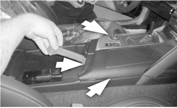
40. Put the shifter in 4th gear, then use a plastic trim tool to separate the back and sides of the console panel from the console base.
