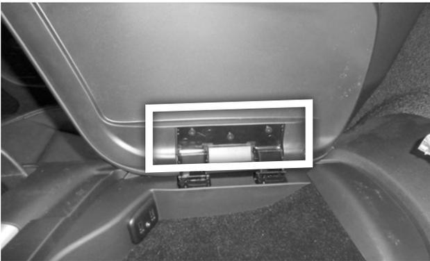
**73. Reinstall the center console lid with its 3 screws**
